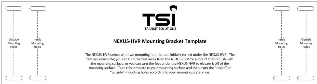
The TSI NEXUS-HVR Mounting Bracket Template is included with every NEXUS-HVR purchase. To use the template, you should tape it to the surface that you will be mounting your NEXUS-HVR on. You can then mark the mounting holes and removed the template, or just drill your holes while the template is taped down.
