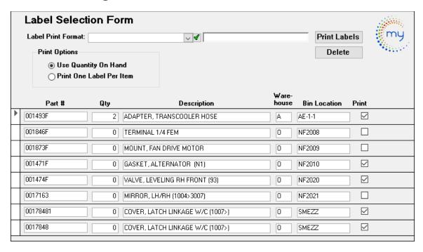
To print labels from the list confirm that the *print check box is checked* and verify the Part # and Qty of labels that will be printed. Next, select the *Label Print Format*
